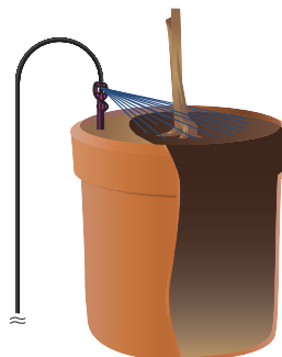
Good Wetting Pattern Even distribution means little or no water and fertilizer will be lost from drainage and the roots will grow evenly throughout.
