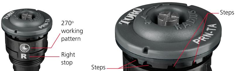
Step-Up™ Technology is designed to deliver high uniformity with matched precipitation for in-close watering all the way out to the furthest radius point. The unique 'steps' create 15 streams, each designed to cover an area of the pattern.
