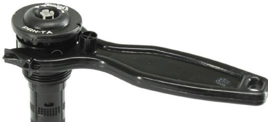
The unique adjustment method allows for pre-setting of arc by hand or tool before the nozzle is installed. Visual indicators allow the user to quickly adjust the arc pattern to the desired arc from 45 - 270°. The adjustment band can be adjusted by hand or with the adjustment tool.
