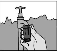
3. Attach the pressure regulator to the garden 4. Screw the 3/4" nut & tail onto the pressure tap (or the tap timer if you have one fitted). Use the tap adaptor if the tap connection is too the tail, securing it with the ratchet clamp. large. NOTE: If the water is non-potable, you may need filtration.
