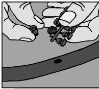
10. If you change your mind about the location of an emitter after punching the hole, insert a Goof Plug to block the opening.
