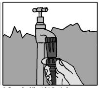
regulator & connect the 13mm poly tube onto TIP: It is easier to push the tube onto fittings if you CAREFULLY dip the end of the tube into a container of hot water for a few seconds.
