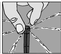
13. Finally, with the water turned on, rotate the cap of each Shrubbler Spike to get the desired wetting performance. You have now successfully installed your Shrubbler Spike system.
