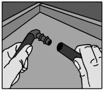
1. Plan your system. Where will you place the 2. Lay out the 13mm poly tube according to your plan. To change direction or add another route, cut the tube and use the elbows and
