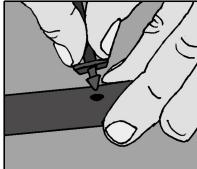
of the adaptor, then push the adaptor into the push it onto the barb on the Shrubbler Spike. hole in the 13mm poly tube.
