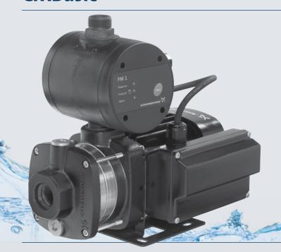
The Grundfos CMBasic is a compact booster pump designed for domestic and light industrial use. The booster unit consists of a Grundfos CM cast iron pump and PM1 pressure manager. The pressure manager allows the pump to start and stop automatically according to demand and protects the pump from dry running.
