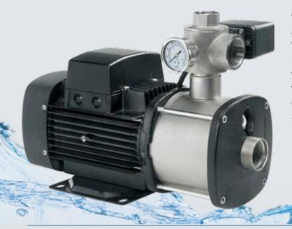
The CM-PS is a compact booster solution designed for domestic and light industrial use. The booster unit consists of a robust CM pump, 5-way valve and a pressure switch. To complete the booster system a pressure tank must be fitted. The pressure switch and pressure tank ensure a convenient water supply with a minimum start/stop frequency.
