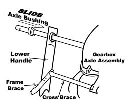
7. Slide axle bushing over axle and into axle bearing to both sides as shown.
