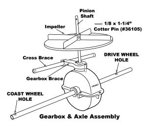
**3.** Install impeller onto pinion shaft. Insert 1/8"x 1¼" cotter pin through impeller then through pinion shaft. Use hole closest to the gear box. Spread cotter pin to prevent from falling out. Next insert Cross Brace thru the Gearbox Brace as shown above.
