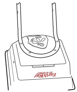
**4.** Install gear box by inserting the pinion shaft into hole in center of hoppers bottom. The word "FRONT" on the gearbox must point to *Front* of the hopper. Follow label instructions on hopper.
