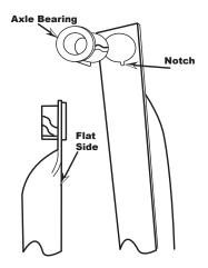
**5.** Install axle bearings to both lower handles. **NOTE:** Notch on bearings and lower handles. Bearings must go through flat side of lower handle.
