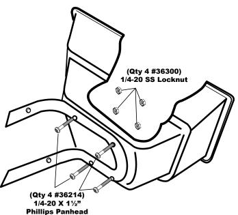
**2.** Position hopper on side. Install frame using (4) 1/4-20 x 1-1/2" Pan Head Phillips bolts and (4) 1/4-20 nylon insert locknuts. First put bolts through holes in frame then through holes in bottom of hopper. Secure with locknuts. **TIGHTEN THESE LOCKNUTS NOW - DO NOT TIGHTEN WITH POWER TOOLS.**
