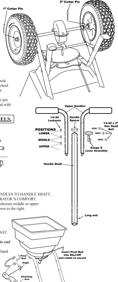
13. Install handle shaft to lower handles and pivot & bracket assembly as shown. Using 1/4 -20 x 2" bolts and locknuts. TIGHTEN BOLTS AND NUTS NOW. 1/4 - 20 Lock-nut <u>a 10</u> Pivot Bracket 1/4 - 20 x 2" Bolt **14.** Install (1) 1/4-20 Hex nut (not a locknut) on to Long End control rod as shown. **Handle Shaft** Holes are farthe from one end Gauge & Lever 30 **Control Rod** Tabbed Hole
