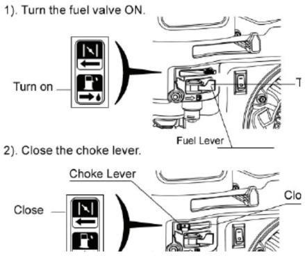
**NOTE:** In case the engine is warm or ambient temperature is high, it's not necessary to close the choke lever.
