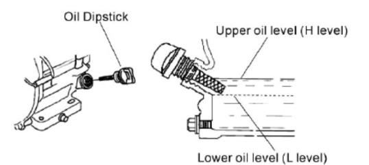
**IMPORTANT:** The Oil Shortage Alarm System is designed to avoid damage of the engine due to shortage of oil in the crankcase. The system will automatically shut down the engine just before the crankcase oil level drops down to the minimum line of safety.
