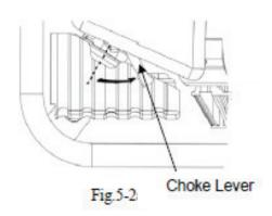
**NOTE:** In case the engine is warm or ambient temperature is high, it's not necessary to close the choke lever. (keep lever to the left)
