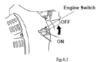
**NOTE:** Turn the engine switch to the OFF position immediately to shut down the engine in an emergency.
