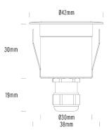
Allow an extra 20mm in height for the cable
